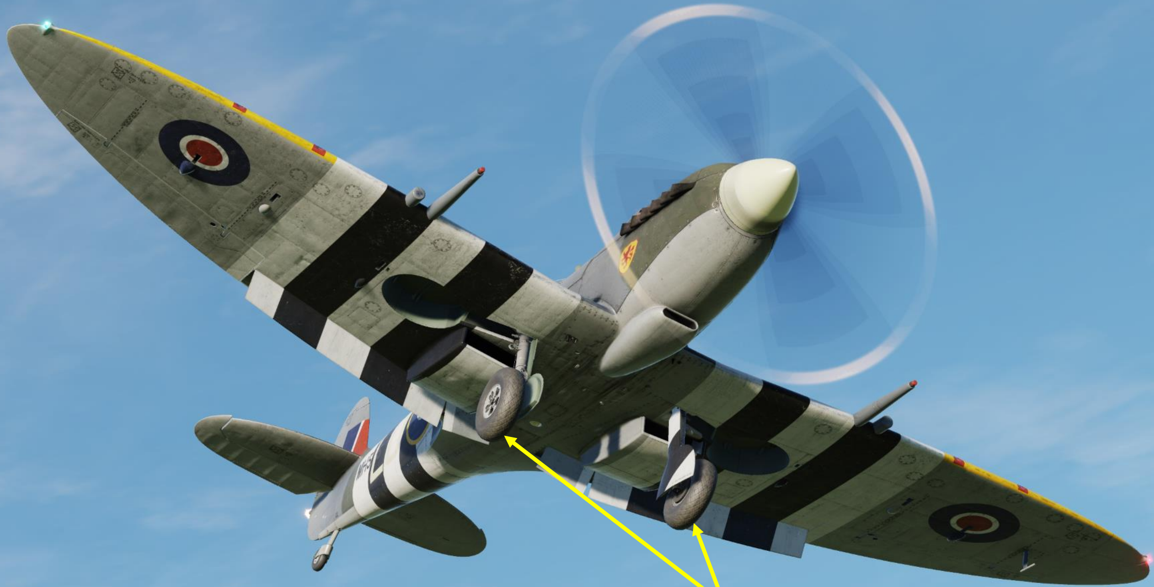
Landing Gear (shown deployed) Hydraulically actuated
